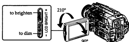
When closing the LCD panel, set it vertically until it clicks, and swing it into the camcorder body.
