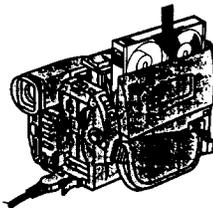
3 Close the cassette compartment by pressing the "PUSH" mark on the cassette compartment. The cassette compartment automatically goes down.
