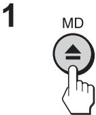
Press **▲ MD** to open the operating panel (or touch **▲** on the main unit) and insert a recordable MD to be recorded into the slot.
