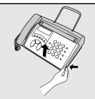
**2** Flip up the green levers on each side of the white roller.
