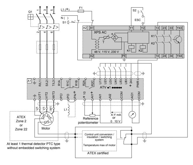
Note: Use cable ends DZ5CE020 (Yellow) on wires connected to PWR and +24 inputs.
