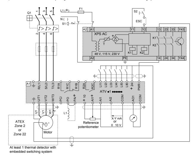
Note: Use cable ends DZ5CE020 (Yellow) on wires connected to PWR and +24 inputs.
