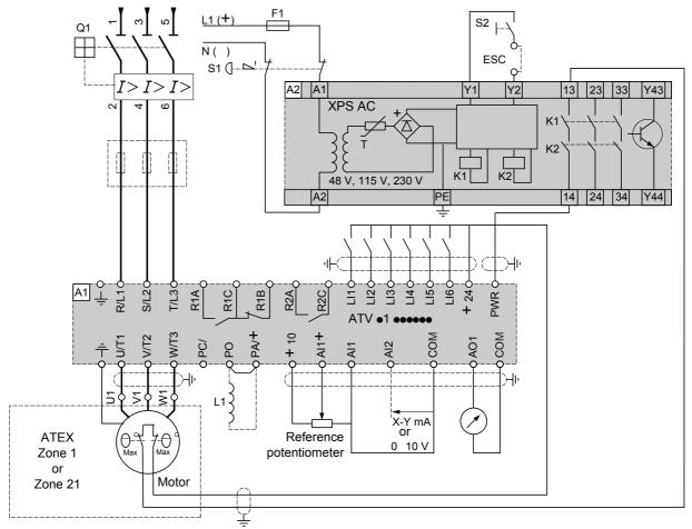
At least 2 thermal detectors with embedded switching system
