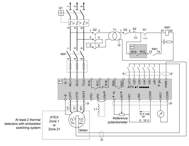
Note: Use cable ends DZ5CE020 (Yellow) on wires connected to PWR and +24 inputs.
