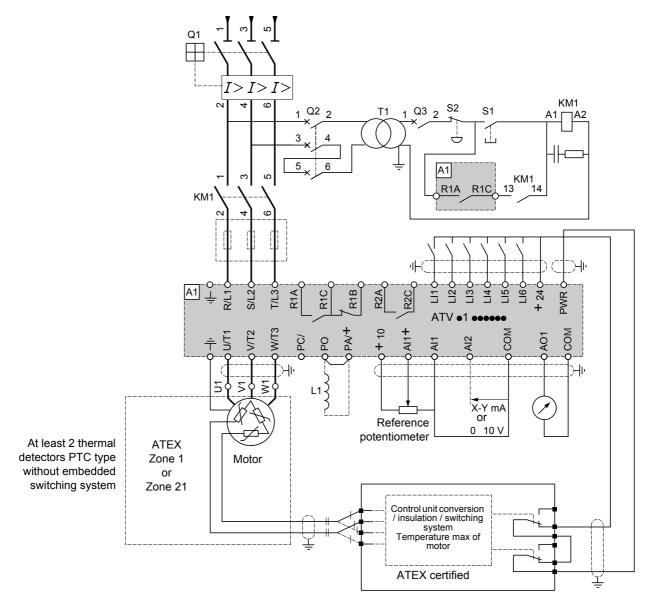
Note: Use cable ends DZ5CE020 (Yellow) on wires connected to PWR and +24 inputs.
