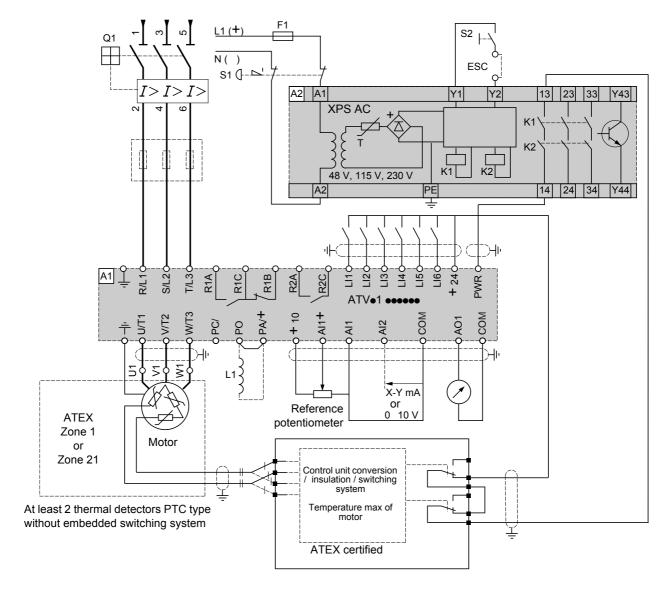
Note: Use cable ends DZ5CE020 (Yellow) on wires connected to PWR and +24 inputs.
