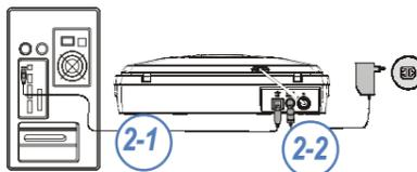
With the power to your PC on, connect the scanner's USB cable to the USB port of your PC (2-1). Connect the power adapter to the scanner and plug it into an appropriate power outlet (2-2).
