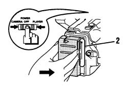
**To remove the battery pack,** push and hold down the **BATT** button, then slide the battery pack in the opposite direction of the arrow on the battery pack ( $\triangleright$ ).
