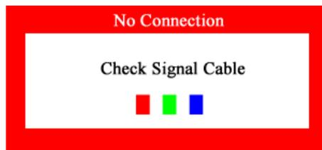
Failure of any of the boxes to appear indicates a problem with your monitor. This box also appears during normal operation if the video cable becomes disconnected or damaged.
