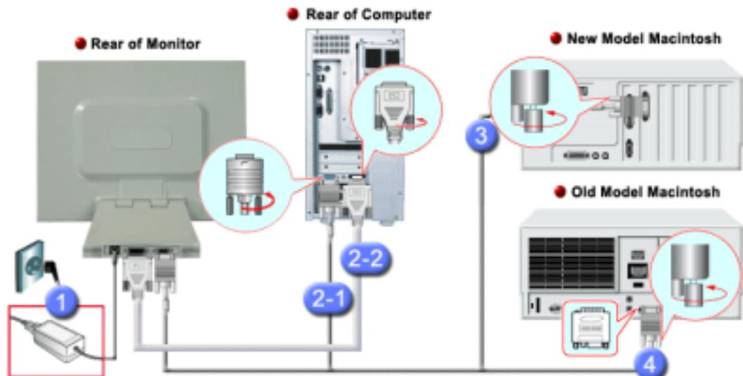
1. Connect the DC Adapter for your monitor to the power port on the back of the monitor. Plug the power cord for the monitor into a nearby outlet.
