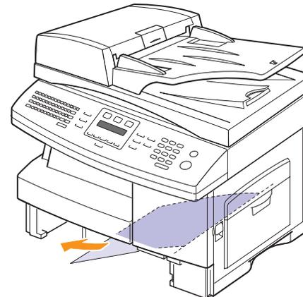
Once you remove the jammed paper here, open the side cover and then close it to clear the "Paper Jam0" message on the display.
