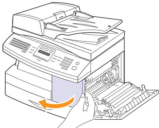
3 Pull down on the fuser lever. This will release pressure on the paper.
