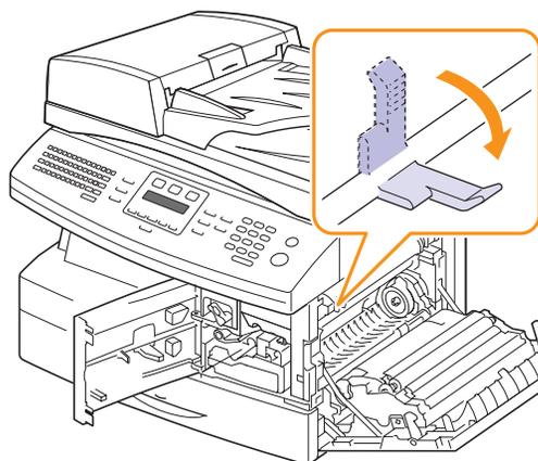
4 Turn the Jam Remove Lever in the direction of the arrow to move the paper to the exit area, then gently pull the paper out through the exit area.
