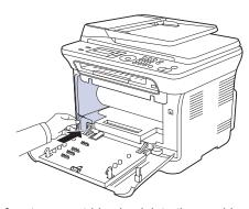
9. Slide four toner cartridge back into the machine.
