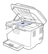
Do not touch the fuser inside the inner cover. It is hot and could cause burns! The fuser's operating temperature is  $180^{\circ}$ C ( $356^{\circ}$ F). Take care when removing paper from the machine.
