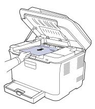
8. Lowering down the scan unit gently and slowly until it is completely closed. Make sure that it is securely latched.
