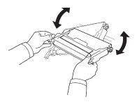
**6.** Place the toner cartridge on a flat surface, as shown, and remove the protecting cover.
