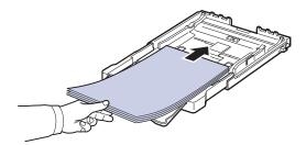
4. Slide the paper length guide until it lightly touches the end of the paper stack. Squeeze the paper width guide and slide it to the edge of the paper stack without causing it to bend.
