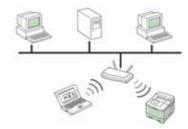
If you know that you are connecting to an Infrastructure mode network with an access point, and the IP address is assigned by a DHCP server, you may proceed to the **Configuring the machine's wireless network** part after reviewing the following parts on printing a **Network Configuration Report**.
