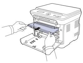
4. Pull the waste toner container out of the machine using its handle.
