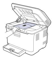
Do not touch the fuser inside the inner cover. It is hot and could cause burns! The fuser's operating temperature is 180°C (356°F). Take care when removing paper from the machine.
