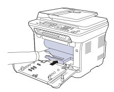
**8.** Insert the waste toner container into position and then push it to make sure that it is firmly seated in place.
