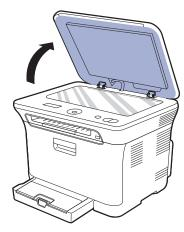
2. Place the original face down on the scanner glass and align it with the registration guide at the top left corner of the glass.
