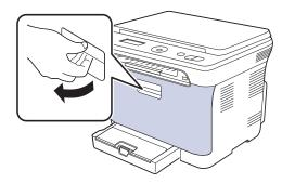
Grasp the handles on the toner cartridge and pull to remove four cartridges from the machine.
