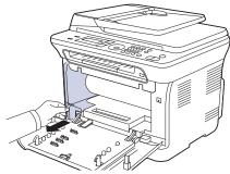
5. Pull the imaging unit out of the machine using the groove on the front of the imaging unit.
