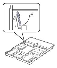
3 Squeeze the paper width guide and slide it to the edge of the lever.
