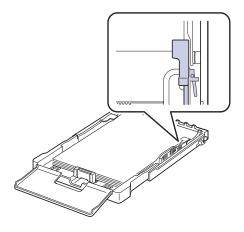
If you want to change the size to A4, first move the paper width guide to left and rotate the lever counterclockwise. If you force the lever, it could damage the tray.
