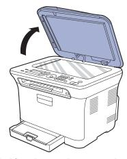
2. Place the original face down on the scanner glass and align it with the registration guide at the top left corner of the glass.
