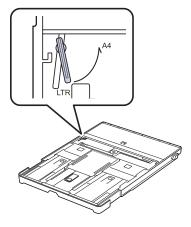
3 Squeeze the paper width guide and slide it to the edge of the lever.
