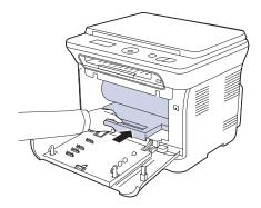
**8.** Insert the waste toner container into position and then push it to make sure that it is firmly seated in place.
