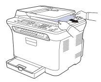
3. Load the removed pages back into the ADF.
