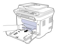
**6.** Take a new imaging unit out of its package. Remove the protective devices on both sides of the imaging unit and the paper protecting the surface of the imaging unit.
