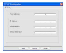
MAC Address: Find the machine's MAC address from the Network Configuration Report and enter it without the colons.
