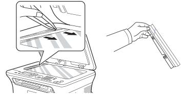
**6.** Hold the edge of the ADF sheet, and wipe both sides of the ADF sheet until it is clean and dry.
