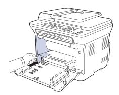
9. Slide four toner cartridges back into the machine.
