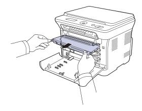
4. Pull the waste toner container out of the machine using its handle.
