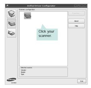
When you have only one MFP device and it is connected to the computer and turned on, your scanner appears on the list and is automatically selected.
