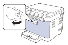
3. Pull the waste toner container out of the machine using its handle.
