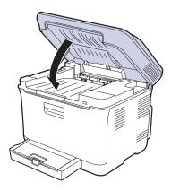
⚠ If the scan unit is not completely closed, the machine will not operate.
