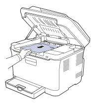
**8.** Lowering down the scan unit gently and slowly until it is completely closed. Make sure that it is securely latched. Be careful not to pinch your fingers!
