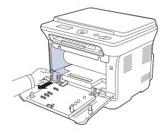
5. Pull the imaging unit out of the machine using the groove on the front of the imaging unit.
