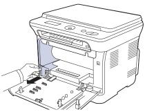
5. Pull the imaging unit out of the machine using the groove on the front of the imaging unit.
