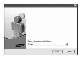
The window above may slightly differ, if you are reinstalling the driver. 5. Select Typical installation for a network printer, and then click Next.
