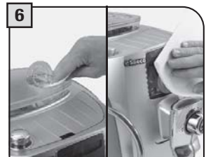
Clean the pre-ground bypass doser with a dry cloth. Wipe the display.
