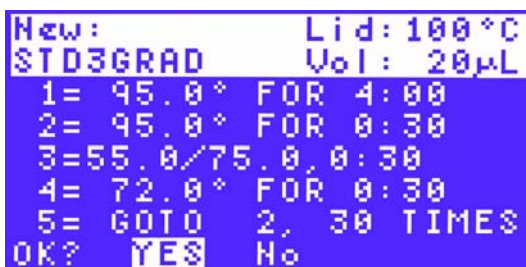
Figure 27. Confirm a GOTO step by selecting YES.
