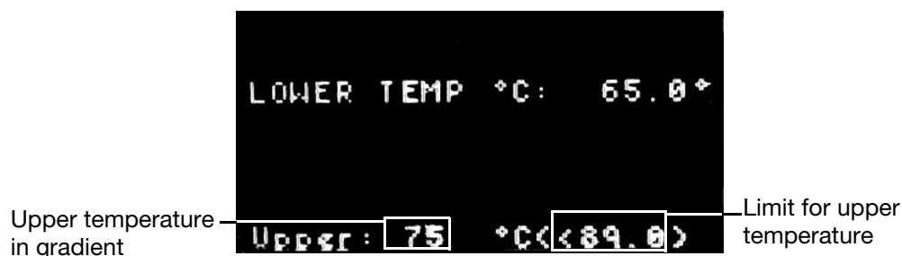
Figure 96. Enter the upper temperature in the gradient.
