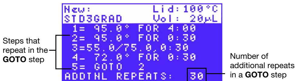
Figure 26. Enter the number of repeats in a GOTO step.
