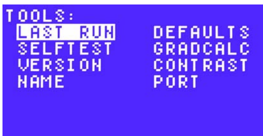
Figure 83. Select LAST RUN for a summary of the last protocol run on the cycler.
