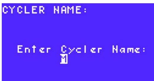
Figure 90. Enter the new thermal cycler name one character at a time.
