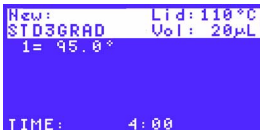
Figure 19. The hold time is 4 minutes in this protocol.
