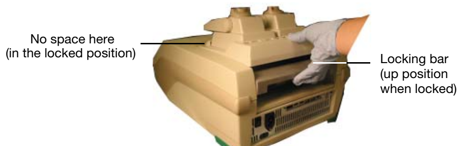
Figure 7. Locking the reaction module in place.
