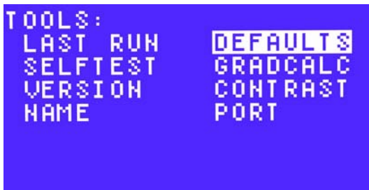
Figure 92. Select DEFAULTS to change the default parameters on the thermal cycler.
