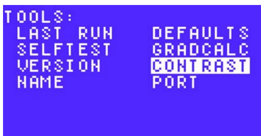
Figure 98. Select CONTRAST to change the contrast of the LCD.
