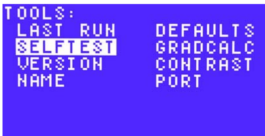
Figure 85. Select SELFTEST to manually run a self test.
