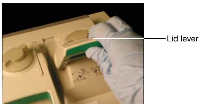
Figure 11. Push the lid lever down.
