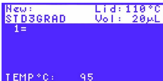
Figure 18. Target temperature of 95°C is used in this protocol.
