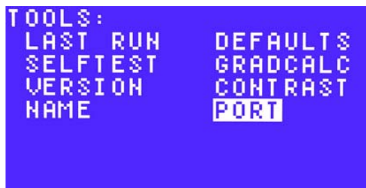
Figure 100. Select PORT to set up the S1000 thermal cyclor for remote control.
