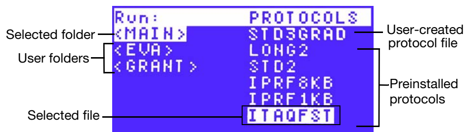
Figure 14. The file tree of the S1000 thermal cyclers.
