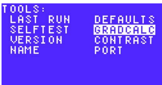
Figure 94. Select GRADCALC to view the temperature in each row of the block.
