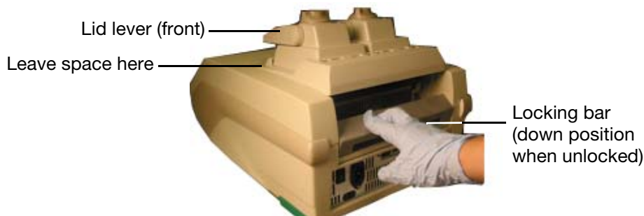
Figure 6. Inserting the reaction module into the bay.
