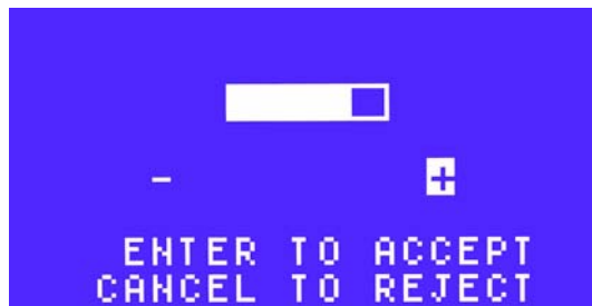
Figure 99. Increase the contrast using the right arrow key.
