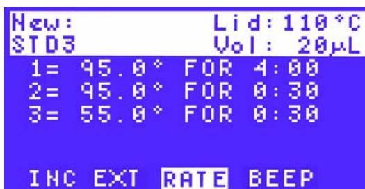
Figure 34. Select RATE to change the ramp rate.
