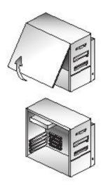
Select an available PCI slot and, if necessary, remove its cover plate. Keep the mounting screw to secure your sound card later. Save the mounting plate for possible use later.
