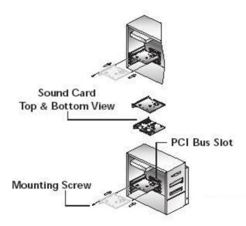
Align sound card and fit firmly into
