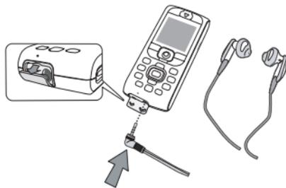
*The headset is activated by default and is also used as the radio antenna. This is why you MUST plug in the headset to listen to the radio, even when using the loudspeaker.*
