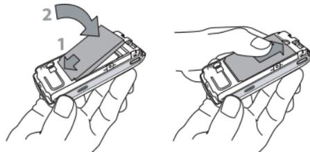
4. Replace the back cover of your phone: hook the front housing onto the hinges on the top of the phone, then press the bottom down until the latch catches.
