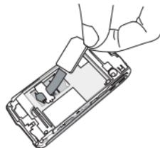
3. Slide the battery door into its slot, metallic connectors downwards, until it stops. Then lock it by pushing it downwards.
