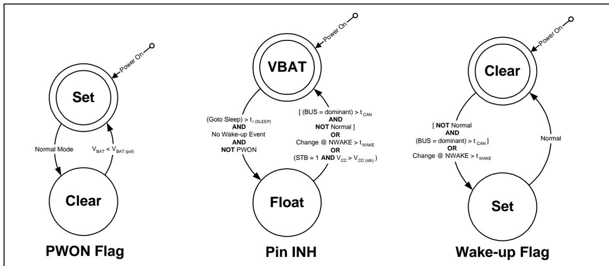
Figure 4 : State Diagrams, PWON Flag, pin INH and Wake-up Flag
