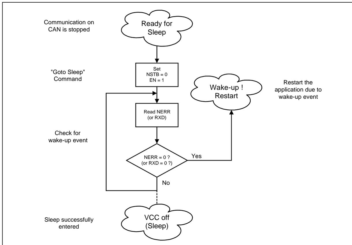
Figure 9 : Software Flow Example, Sleep Mode
