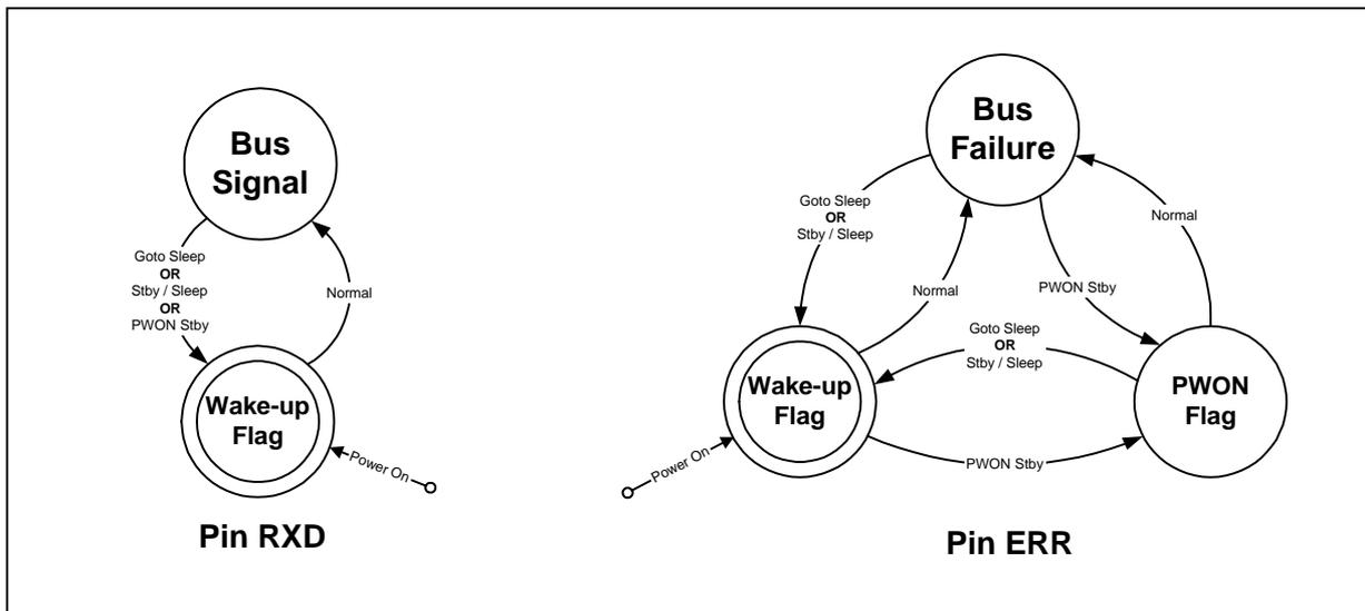
**Figure 5 : State Diagrams, pins RXD and ERR**
