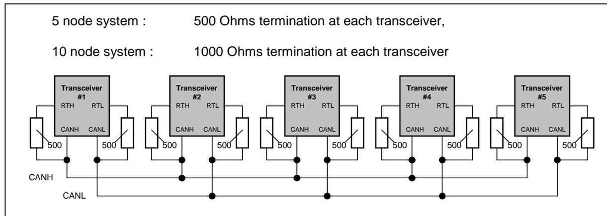
Figure 6 : Example Network with 5 nodes, 500 Ohms termination at each node
