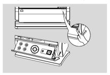
2 Insert the USB device's USB plug into the socket on the set's foldable control panel
