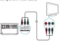
Connect a progressive scan TV through component video cables for higher quality video.
