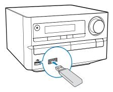
1 Press **USB** to select the source for USB storage device.
