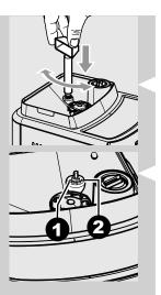
coffee bean hopper. This must be pressed and turned using the supplied key only.
