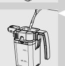
2 Pour the milk: The level of milk poured into the carafe must be between the (MIN) level and the (MAX) level.
