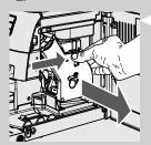
4 Remove the brew group: Pull it by the handle and press the «PUSH» button. The brew group must be washed only with lukewarm water with no detergent.
