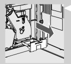
4 When emptying the coffee grounds drawer it is also necessary to empty and clean the coffee residues drawer. Open the service door, remove the drawer and empty the coffee grounds.
