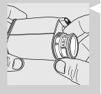
3 The filter should be set according to the measurements performed to set the water hardness. Use the water hardness test strip provided with the machine. Set the "Intenza Aroma System" as specified on the filter packaging (see section "Measuring Water Hardness").
