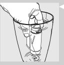
Remove the "INTENZA+" water filter from its packaging, immerse it vertically (with the opening positioned upwards) in cold water and delicately press the sides so as to let the air bubbles out.
