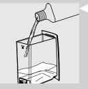
4 Pour the entire content of Saeco concentrated descaling solution into the appliance water tank.
