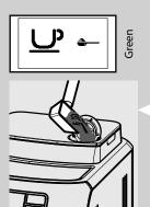
Warning: Add only pre-ground coffee to the compartment. Other substances and objects may cause severe damages to the machine. Such damages will not be covered by warranty.
