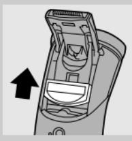
**1** Open the trimmer by pushing the slide upwards.
