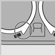
**4** Remove the shaving heads and place new ones in the shaving unit in such a way that the projections fit exactly into the recesses in the shaving unit.
