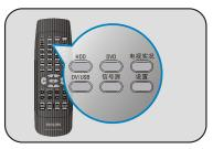
4C To select recording media. Press DVD REC repeatedly to select "Rec to: Optical disc" or "Rec to: Hard disc". Press ADD/CLEAR to toggle between the different modes of record quality.
