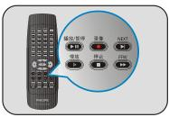
4 To pause the recording, press PLAY/PAUSE. Press REC to resume recording and press STOP key to stop recording.
