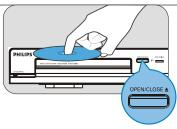
4a Press OPEN/CLOSE ▲ to open the disc tray, load a recordable DVD±R/±RW with the label facing up.
