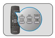
4 To select external program source. Press SOURCE repeatedly to select the source to record from. Input Source: CAM 1, R CVBS, R Y/C, R YUV, CHXXX or press DV/USB twice to select input source of DV.
