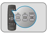
Press TUNER, then press CH+ and CH- keys to select a TV channel. Press HDD to access to title recordings in hard disc. Press DVD to access to title recordings in disc.
