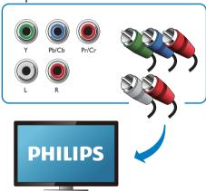
Connect a progressive scan TV through component video cables for higher quality video.
