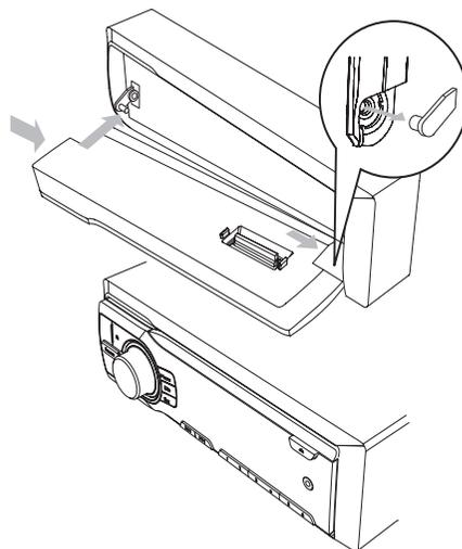
2 Insert the right side of the panel in the chassis until it is correctly engaged.
