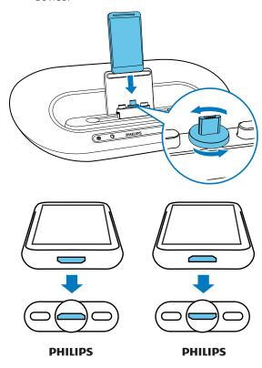
2 Slide the connector to the center of the device.
