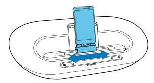
**3** Adjust the bumpers on both sides to stabilize the portable device.
