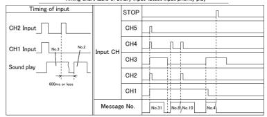
6-5-7.Bit input hold play mode(operation mode switch: G)
