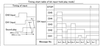
6-5-8.Binary input hold play mode (operation mode switch:H)
