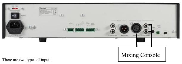
One is balanced signal, the other is unbalanced.
