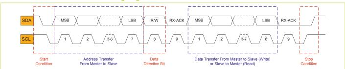
NXP's I<sup>2</sup>C-bus GPIO expanders support three operating modes for data transfer: Standard Mode, with data transfer rates from 0 kbps to 100 kbps, Fast Mode (Fm), with data transfer rates from 0 kbps to 400 kbps, and Fast-mode Plus (Fm+) with data rates from 0 kbps to 1 Mbps. Since the newer Fm+ GPIO are backward compatible all the way back to Standard Mode, it's easy to expand existing designs without changing the bus master device.
