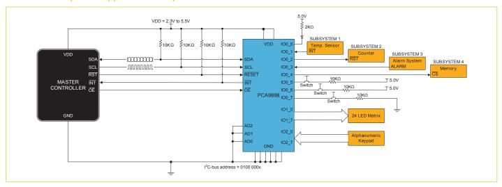
The  $I^2$ C-bus allows easy two-line communication between two devices using a serial data line (SDA) and a serial clock line (SCL) and, as a result, is a popular choice for computing, consumer electronics, communication, and industrial systems.
