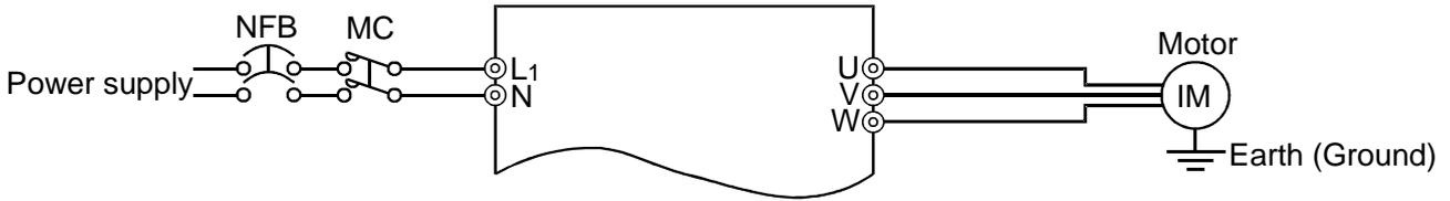
Note: 1. To ensure safety, connect the power input to the inverter via a magnetic contactor and earth leakage circuit breaker or no-fuse breaker, and use the magnetic contactor to switch power on-off.
