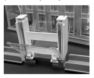
c. Lift the gel sandwiches or cassettes into place against the green gaskets. Make sure the Mini-PROTEAN 3 short plates sit just below the notch in the gasket.
