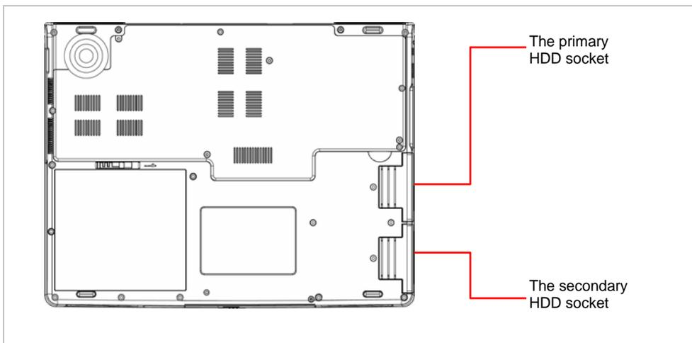
Your **notebook** is equipped with two sets of HDD sockets. These sockets support industry standard 2.5"/9.5mm SATA-2 Gen1i (1.5Gb/s) hard disk drives. Unless you are going to install two Windows bootable HDD drives into these sockets, there is generally no need to distinguish which socket is the **primary socket** and vice versa. Below are the three major scenarios:
