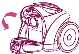
2 Detach the protection filter of the motor from the body after disassembling the dust box.
