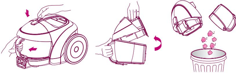
**1** Detach the dust tank when press the button.
