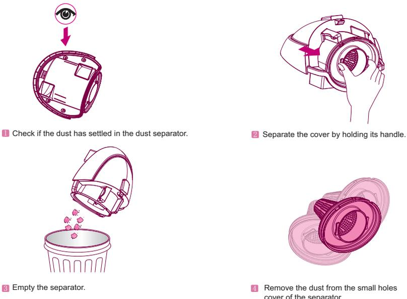
**1** Check if the dust has settled in the dust separator.
