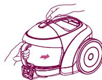
4 Assemble the dust tank.
