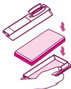
1 Put the filter into the case.
