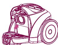
3 Fix the assembled filter.
