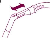
The flexible hose handle has a manual air flow regulator which allows you to briefly reduce the suction level.
