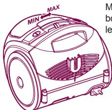
Move the regulator on the body to adjust suction power level .
