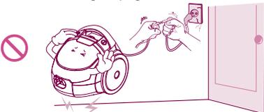
In winding the power cord, hold the plug before pressing the button of the cord reel. Do not pull the power cord beyond the red warning line, other wise the power cord may be damaged or unable to be wound up. Pay attention to the plug in winding the cord to avoid damaging the surrounding objects.
