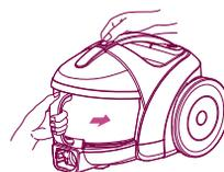
4 Assemble the dust tank.
