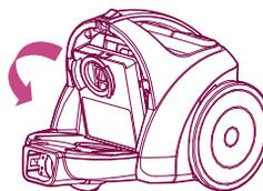
2 Detach the protection filter of the motor from the body after disassembling the dust box.
