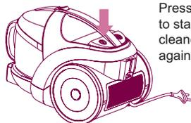
Press power switch to start the vacuum cleaner, press once again to turn off it.
