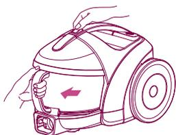
1 Detach the dust tank when press the button.
