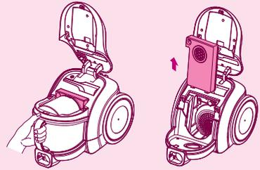
**2** Detach the protection filter of the motor from the body after disassembling the dust box.
