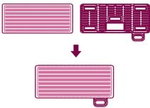
2. After the mop nozzle matches with the mop board, connect the mop nozzle from the top down. When you hear a sound of Ta Ta, it means the connection is ok.
