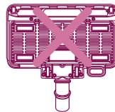
When the mop is not used, you couldn't use the method showed on the left diagram. If not, the mop nozzle will damage the attaching location of mop.
