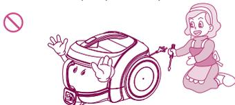
Do not pull or carry by cord, use cord as a handle, close door on cord or pull cord around sharp edges or corners. Do not run appliance over cord. Keep cord away from heated surfaces.
