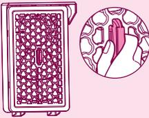
**3** Separate the filter from the cover by holding the handle of the case.
