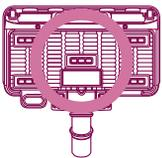
To protect the attaching location of mop, it is recommend connect the mop nozzle according to the left diagram when mop is not used.
