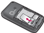
To remove the USIM card
