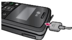
1. With the arrow facing you as shown in the diagram push the plug on the battery adapter into the socket on the left side of the phone until it clicks into place.
