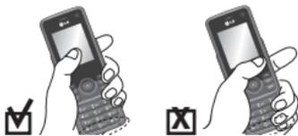
Please do not cover the antenna area with your hand during a call or when using a Bluetooth connection. It may reduce signal quality.
