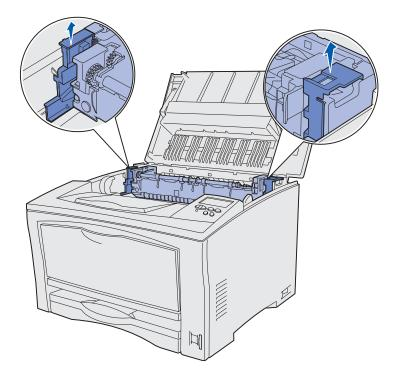
**5** Grasping the handles on each end of the fuser, pull the fuser toward you, and then up out of the printer.
