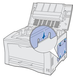
2 Insert the two tabs at the front end of the right cover behind the printer frame, and then align the cover with the release button.
