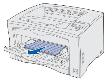
2 If paper is jammed inside the multipurpose feeder, remove it.
