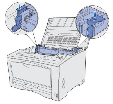
4 Align the print cartridge with the grooves in the printer and reinsert it into the printer.
