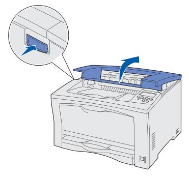
**5** Push the side release button as you slide the right cover toward the rear of the printer.
