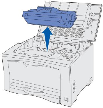
4 Pull up the fuser latches on each end to release the fuser.
