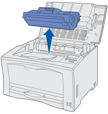
4 Open the print cartridge paper guide lever and remove any jammed paper.
