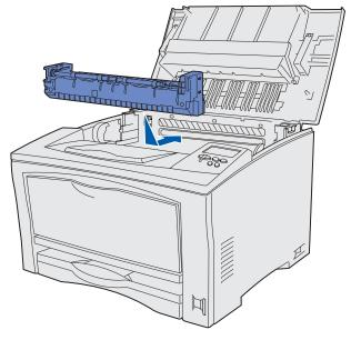
**3** Push down the fuser latches to lock the fuser into position.
