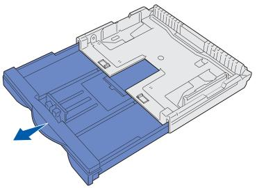
5 Slide the locking mechanisms outward to lock the extension in place.
