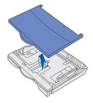
**3** Squeeze the front guide lever and slide the guide to the front of the tray.
