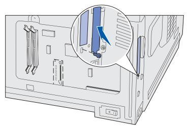
8 Reinstall the access panel (see Reinstalling the system board access panel).
