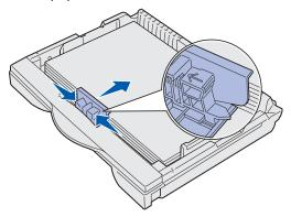
**WARNING:** Do not exceed the maximum stack height indicated on the tray. Overfilling the tray may cause jams.
