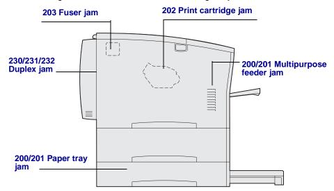
A 200 Paper Jam may occur when the printer is turned off while a job is printing. A 201 Paper Jam occurs when paper does not feed correctly from the tray or multipurpose feeder.
