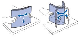
Do not fold or crease the paper. Straighten the edges of the stack on a level surface.
