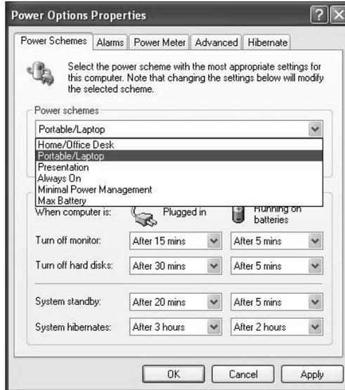
In this dialog box, you can manually set the LCD and hard drive's time-out values in the Plugged in column and in the Running on batteries column. Lower time-out values will save more battery power.
