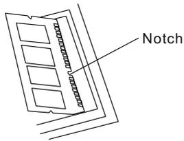
7. Pivot the DIMM until the latches on both sides of the socket snap into place.
