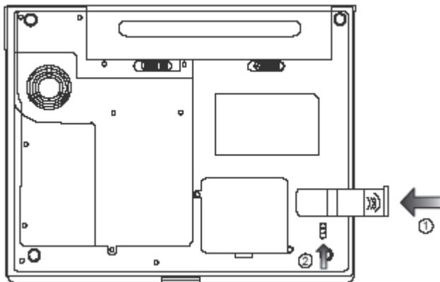
You may install the optional wireless LAN module into this slot.
