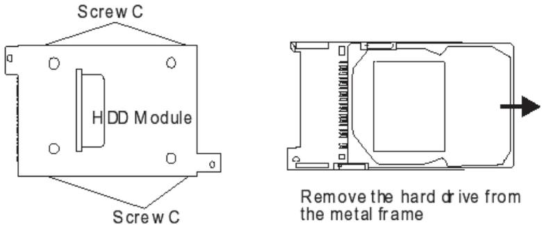
11. Re-attach the metal cover to the new hard drive and tighten 4 Screw C's. Note the green PC board of the hard disk drive is facing against the metal case.
