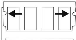
6. Install the new DIMM module into the memory socket. The DIMM will only fit in one orientation. Insert the DIMM at an angle of approximately 30 degrees into the empty memory socket. Then press it firmly so that the contact edge is driven into the receiving socket.
