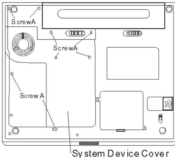
5. In order to prevent the collision with the thermal module when the HDD is being removed, three screws fixed to the thermal module need to be removed first.
