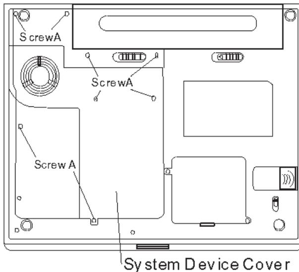
4. Remove the System Device Cover. The DIMM socket is now seen as shown below.
