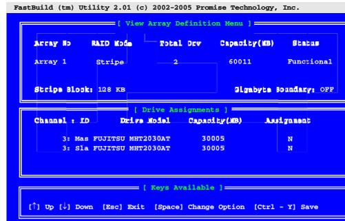
18. First assign the type of **RAID Mode** you want to use by using the <Spacebar> to cycle through the array types (**Stripe** or **Mirror**).
