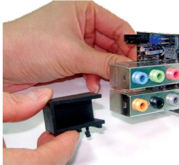
2. Align the module's plugs above the mounting holes then insert the plugs from the top through to the bottom of the system board. While at it, the 14-pin connector at the solder side of the module must also insert into the Karajan audio connector at location J7 of the system board. Make sure the plugs snap firmly out the bottom of the board.
