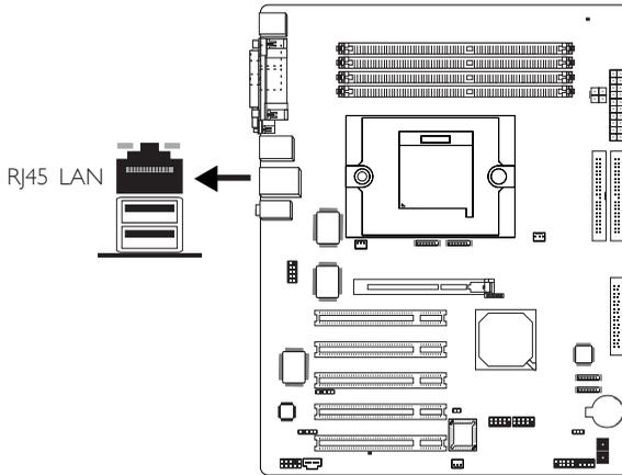
The system board is equipped with an onboard RJ45 fast-ethernet LAN port at location CN4 of the system board. It allows the system board to connect to a local area network by means of a network hub.
