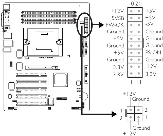
Use a power supply that complies with the ATX12V Power Supply Design Guide Version 1.1. An ATX12V power supply has a standard 20-pin ATX main power connector and a 4-pin +12V power connector that must be inserted onto J24 and CN10 connectors respectively.
