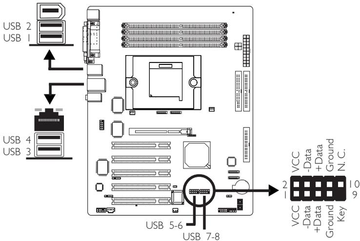
Four onboard USB 2.0/1.1 ports (Black) are at locations CN3 (USB 1-2) and CN4 (USB 3-4) of the system board.
