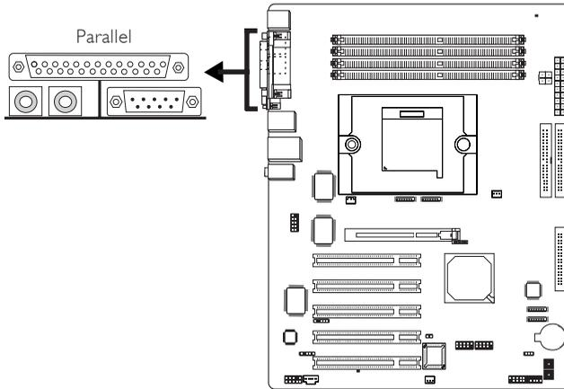
The system board has a standard parallel port (Burgundy) at location CNI for interfacing your PC to a parallel printer. It supports SPP, ECP and EPP.
