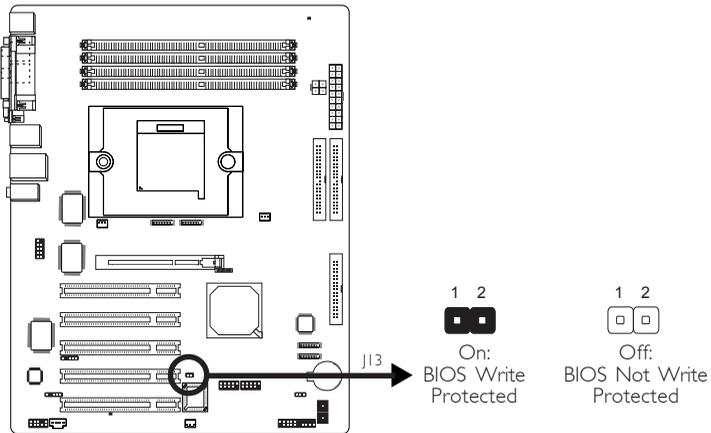
J13 is used to enable or disable the BIOS Write Protect function. When enabled, the system will be protected from unnecessary updating or flashing of the BIOS. It secures the BIOS therefore any updates to it will not take effect.
