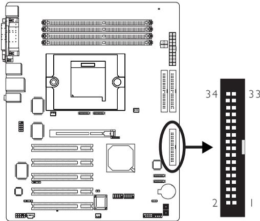
The system board is equipped with a shrouded floppy disk drive connector for connecting two standard floppy disk drives. To prevent improper floppy cable installation, the shrouded floppy disk header has a keying mechanism. The 34-pin connector on the floppy cable can be placed into the header only if pin 1 of the connector is aligned with pin 1 of the header.
