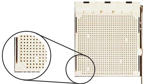
6. Insert the CPU into the socket until it is seated in place. The CPU will fit in only one orientation and can easily be inserted without exerting any force.
