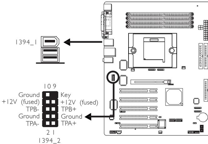
The system board is equipped with an onboard IEEE 1394 port at location CN3 (IEEE 1394\_1) of the system board.
