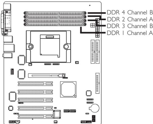
The system board supports DDR SDRAM DIMM. Double Data Rate SDRAM (DDR SDRAM) is a type of SDRAM that doubles the data rate through reading and writing at both the rising and falling edge of each clock. This effectively doubles the speed of operation therefore doubling the speed of data transfer. Refer to chapter 1 (System Memory section) for detailed specification of the memory supported by the system board.
