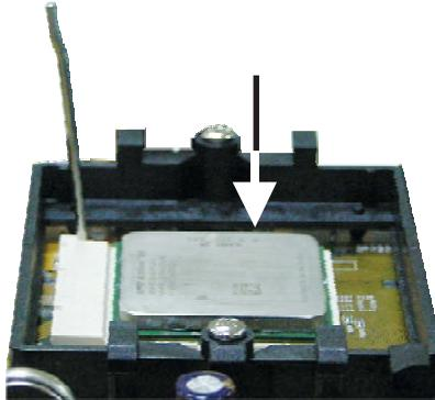
7. Once the CPU is in place, push down the lever to lock the socket. The lever should click on the side tab to indicate that the CPU is completely secured in the socket.
