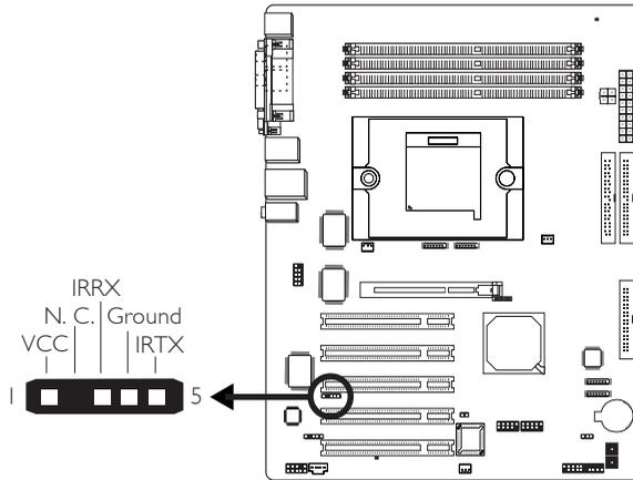
Connect your IrDA cable to connector J5 on the system board.
