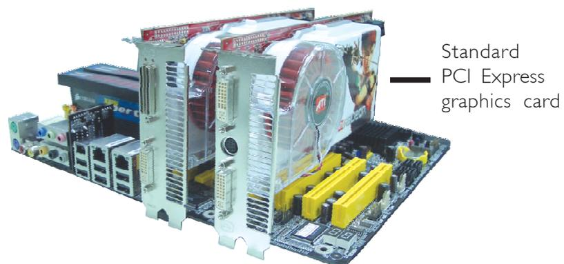
7. Secure the graphics card with the screw you removed in step 5.
