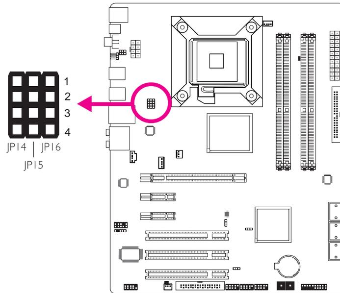
By default, the three jumpers are all set to pins 1 and 2 On. This setting will allow the system to automatically run according to the CPU's FSB. If you want to change the setting, please refer to the table below.
