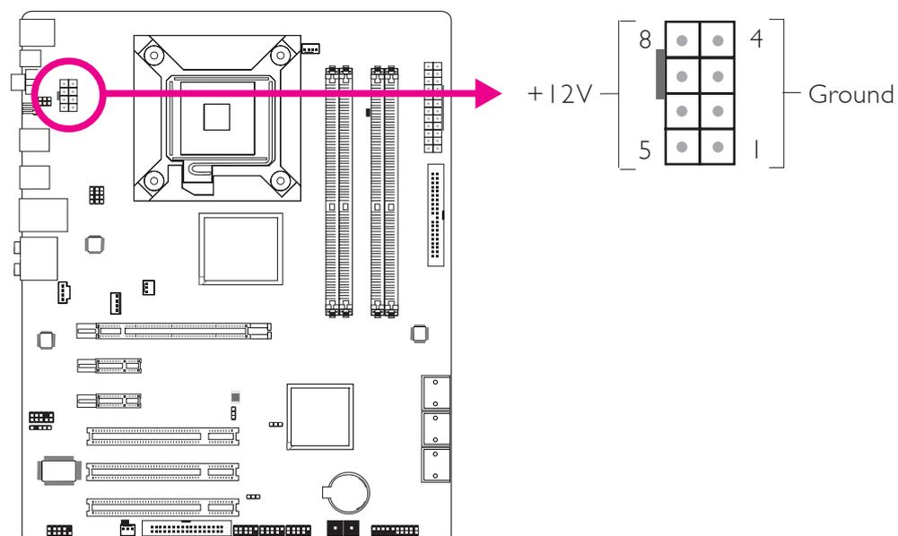
The power connectors from the power supply unit are designed to fit the 24-pin and 8-pin connectors in only one orientation. Make sure to find the proper orientation before plugging the connectors.
