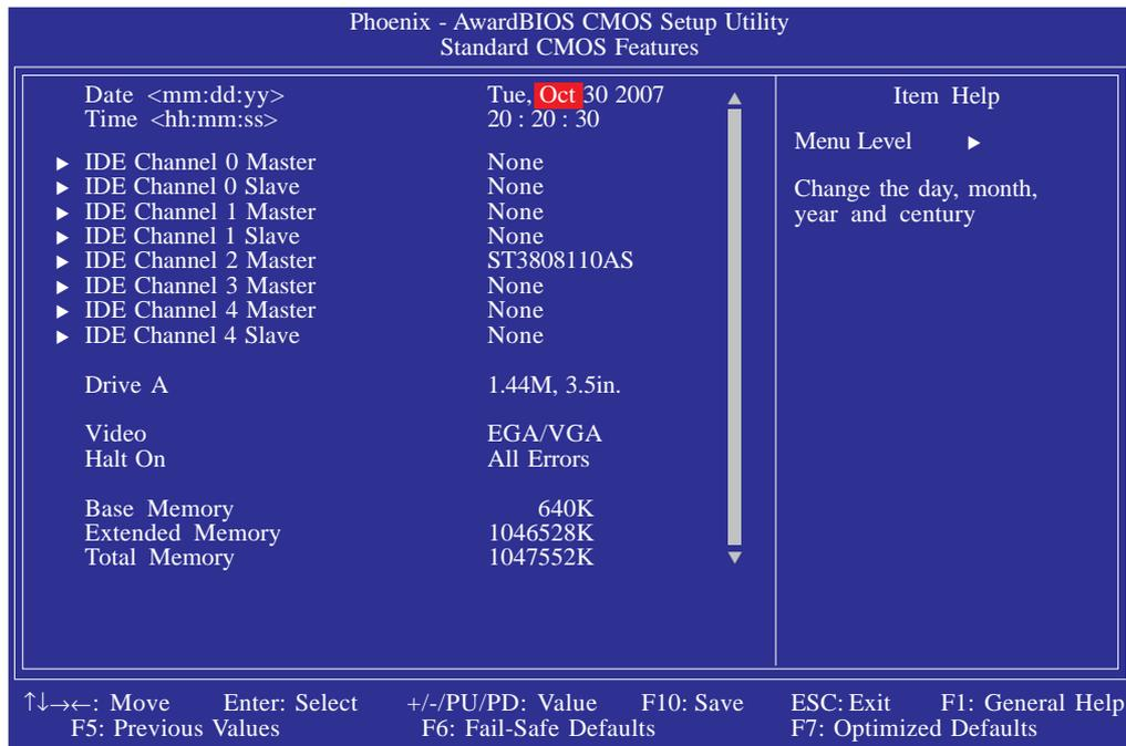
The screen above list all the fields available in the Standard CMOS Features submenu, for ease of reference in this manual. In the actual CMOS setup, you have to use the scroll bar to view the fields. The settings on the screen are for reference only. Your version may not be identical to this one.
