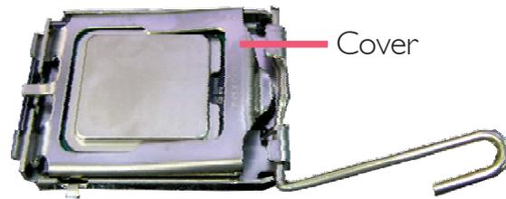
11. Push the lever down to lock the socket. The lever should hook onto the side tab to indicate that the CPU is completely secured in the socket.
