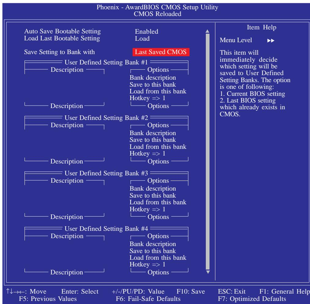
The screen above list all the fields available in the CMOS Reloaded submenu, for ease of reference in this manual. In the actual CMOS setup, you have to use the scroll bar to view the fields. The settings on the screen are for reference only. Your version may not be identical to this one.
