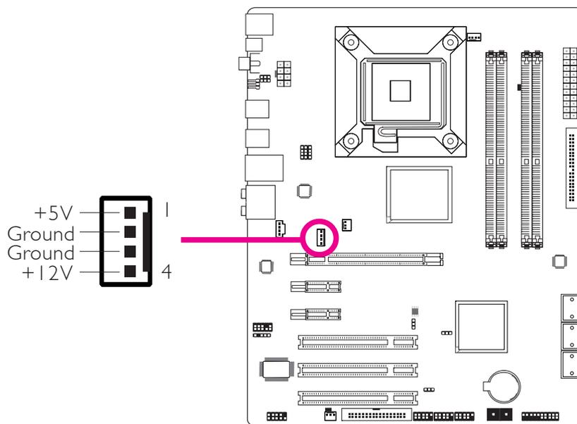
The system board requires a minimum of 300 Watt power supply to operate. Your system configuration (CPU power, amount of memory, add-in cards, peripherals, etc.) may exceed the minimum power requirement. To ensure that adequate power is provided, **we strongly recommend that you use a minimum of 400 Watt (or greater) power supply.**
