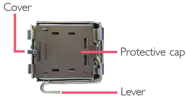
5. Lift the protective cap from the location pointed below to detach the cap from the cover.
