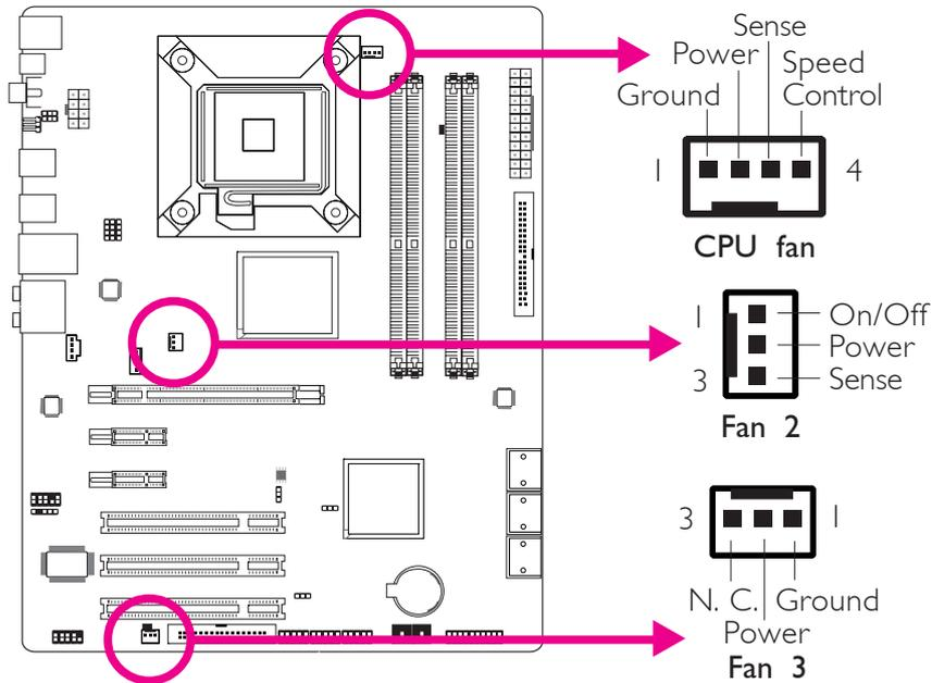
These fan connectors are used to connect cooling fans. Cooling fans will provide adequate airflow throughout the chassis to prevent overheating the CPU and system board components.
