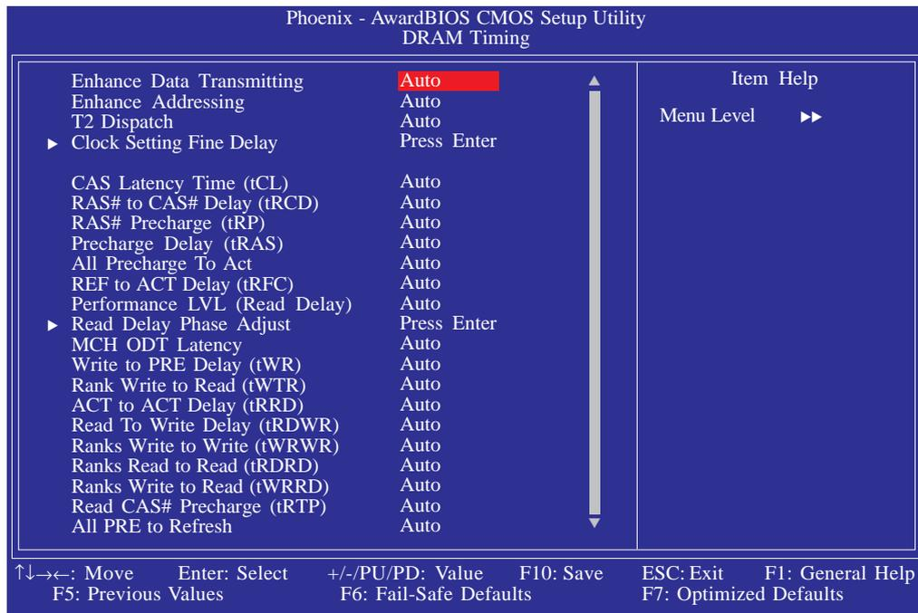
The screen above list all the fields available in the DRAM Timing submenu, for ease of reference in this manual. In the actual CMOS setup, you have to use the scroll bar to view the fields. The settings on the screen are for reference only. Your version may not be identical to this one.
