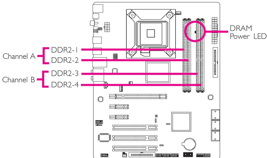
The four DIMM sockets on the system board are divided into 2 channels:
