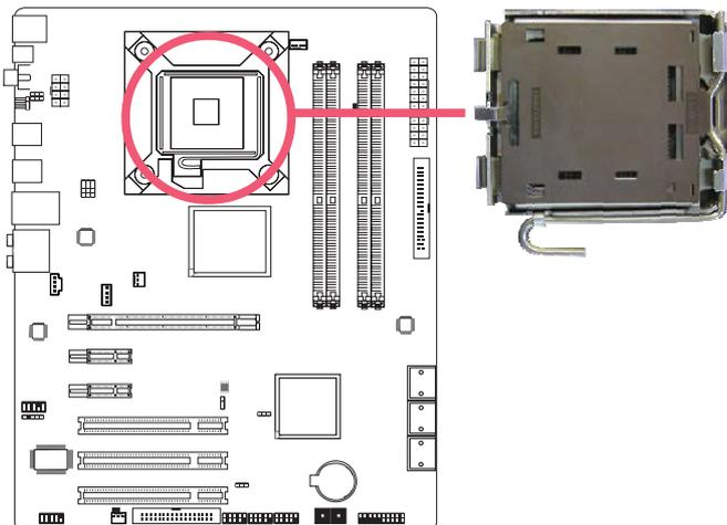
4. The CPU socket comes with a cover that is attached with a removable protective cap. The cap is used to protect the CPU socket against dust and harmful particles. Remove the protective cap only when you are about to install the CPU.
