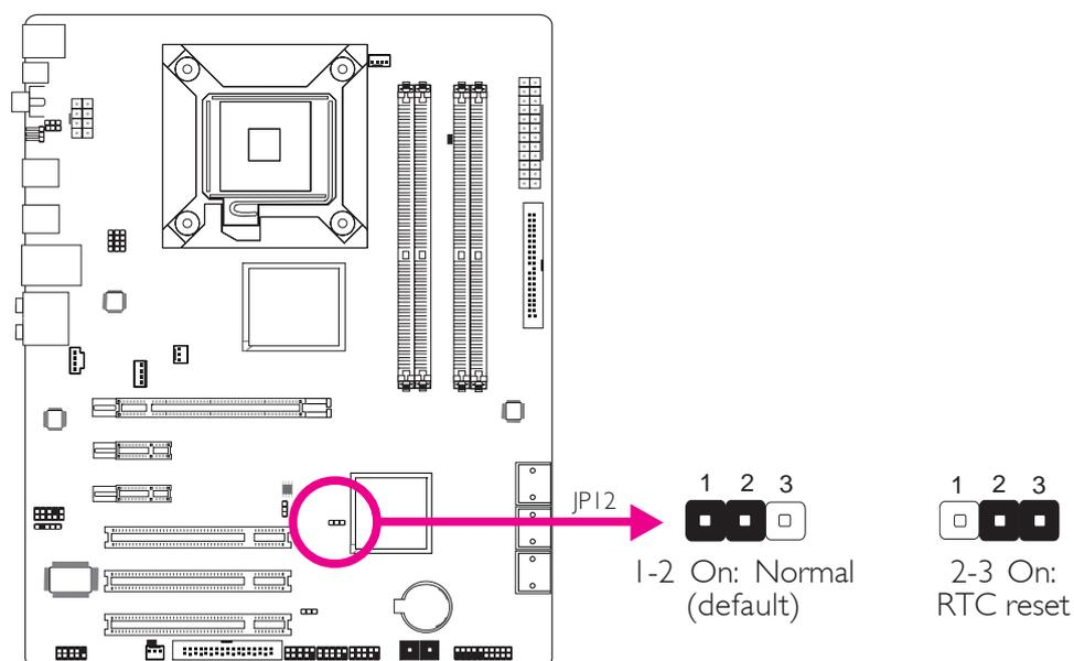
When the RTC battery is removed, this jumper resets the manageability register bits in the RTC.
