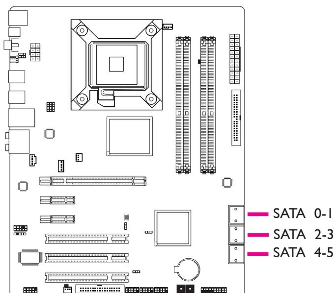
The Serial ATA (SATA) connectors are used to connect Serial ATA drives. Connect one end of the Serial ATA cable to a Serial ATA connector and the other end to your Serial ATA device.
