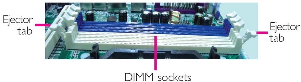
5. Note how the module is keyed to the socket.
