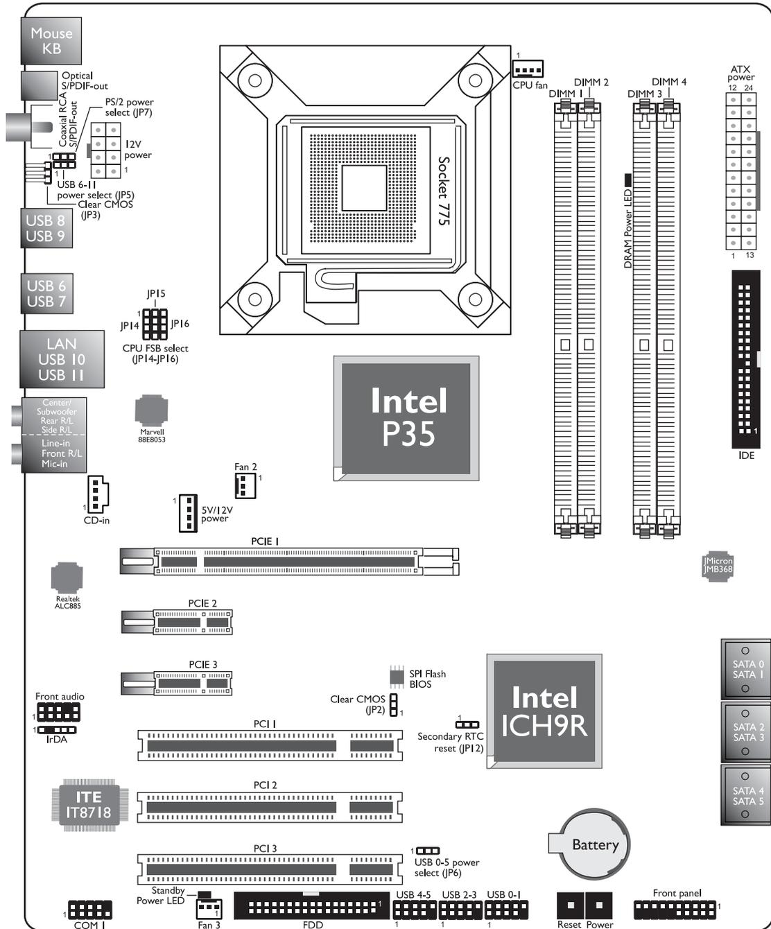
The layout shown above is the LP DK P35-T2RT2RS system board which supports 6 SATA ports. On the LP DK P35-T2 board, it only supports 4 SATA ports (SATA 0/1/4/5).
