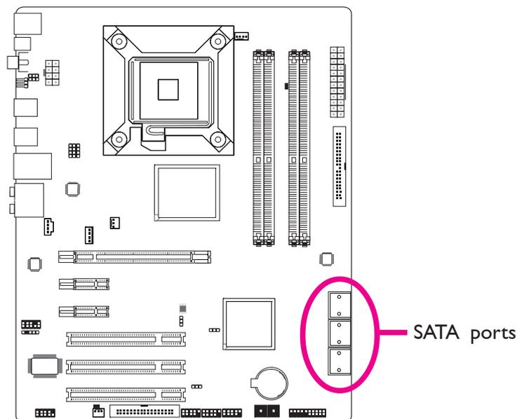
Refer to chapter 2 for details on connecting the Serial ATA drives.
