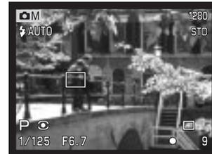
Pressing the shutter-release button partway down (3) or pressing the center of the controller (4) will select the area; the other four areas will disappear.
