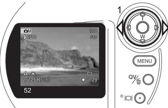
The aperture value can be changed in two steps: f/3.0 and f/6.7 at the lens' wide-angle position, f/3.6 and f/8.0 at the lens' telephoto position. As the lens is zoomed, the aperture will automatically shift. If the aperture value is beyond the shutter-speed range, the shutter-speed display will turn red on the monitor. For more on the aperture and image control, see page 62.
