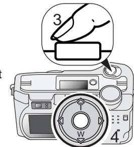
Once a spot focus area is selected, it will remain active even after the picture has been taken. Only when one focus area is displayed, can the controller be used to zoom (p. 22) or adjust the exposure (p. 52).
