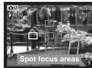
Press and hold the controller to display the spot focus areas; the active area is blue. Use the four-way key of the controller (2) to highlight the desired autofocus area.
