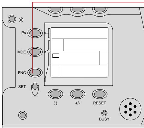
**1** Press and hold the FNC button and rotate the Main-Command dial until the Function Set indicator (▼) appears in the Camera Status LCD panel and **ISO** and **A** (if auto ISO is selected) start blinking.
