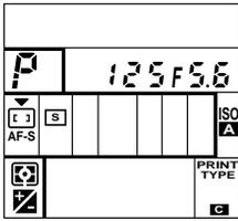
Once set, Exposure Compensation remains fixed until reset. The
