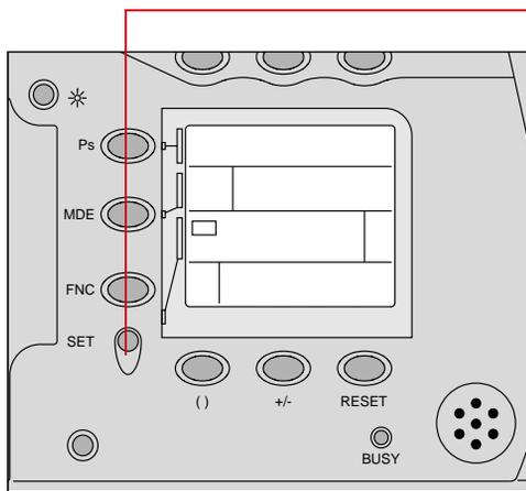
**3** Press and hold the SET button and rotate the Main-Command dial to set for single-frame shooting or for continuous shooting.
