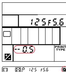
The  $\pm$  symbol appears in the Camera Status LCD panel and inside the viewfinder. (The example at the left shows a -1/2 EV compensation setting.)
