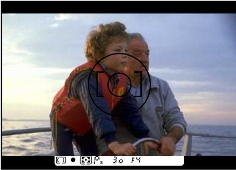
When subject brightness is insufficient, lightly pressing the Shutter Release button to activate the exposure meter also turns on the Flash Recommended light (green ⚡) inside the viewfinder. You can use the built-in flash or Nikon Speedlight anytime, regardless of ambient lighting. If your subject is backlit, for example, you can use the built-in flash to illuminate your subject and fill in shadows.
