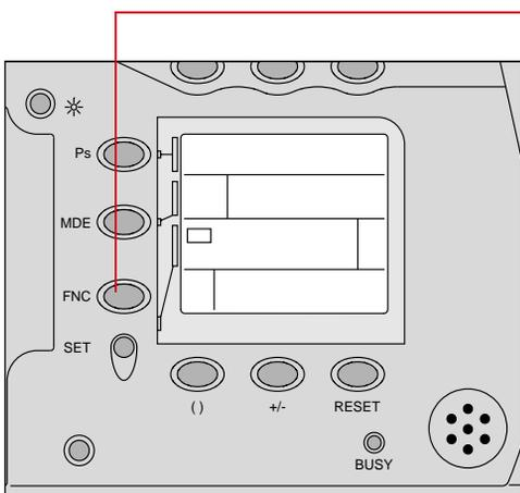
To confirm the compensation value in the Camera Status LCD panel, press and hold the FNC button and rotate the Main-Command dial until the Function Set indicator (▼) appears and
