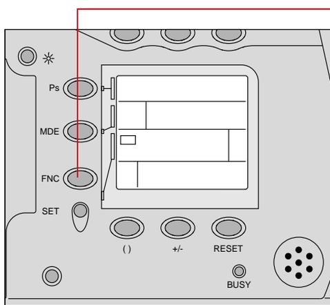
**1** Press and hold the FNC button and rotate the Main-Command dial until the Function Set indicator (▼) appears in the Camera Status LCD panel, and the or symbol starts blinking.
