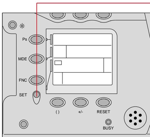
4 Press and hold the SET button and rotate the Main-Command dial until the desired combination appears.
