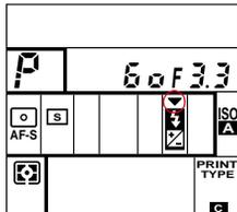
Once set, Flash Output Level Compensation remains fixed until reset. Although ▼ remains in the Camera Status LCD panel to indicate Exposure Compensation is On, the compensation value disappears when you release from the SET button.
