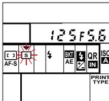
**2** Remove your finger from the FNC button and confirm that the or symbol stops blinking.
