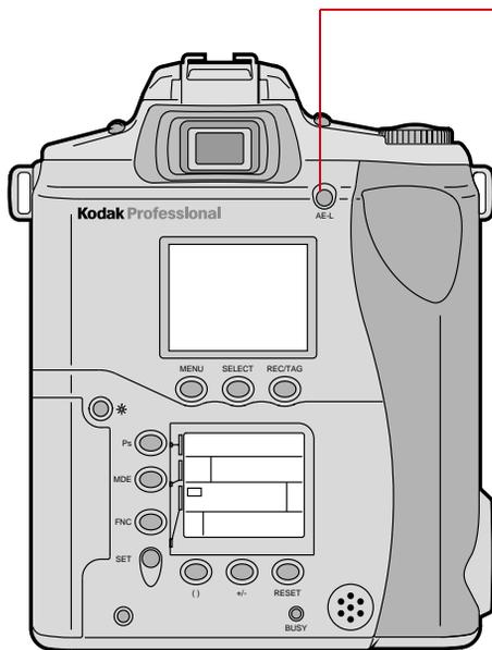
**3** Press and hold the AE-L button to lock auto exposure.
