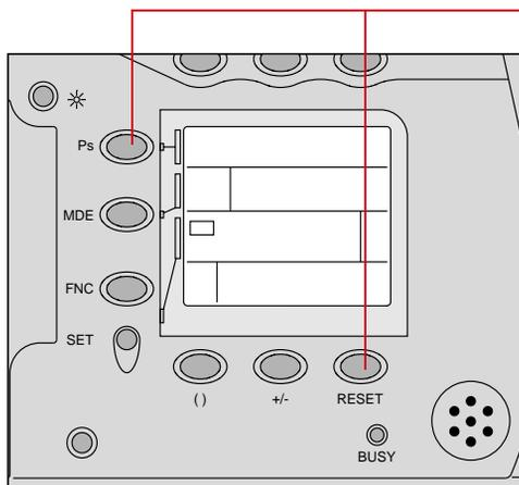
Press and hold the Ps and the RESET buttons for more than two seconds.
