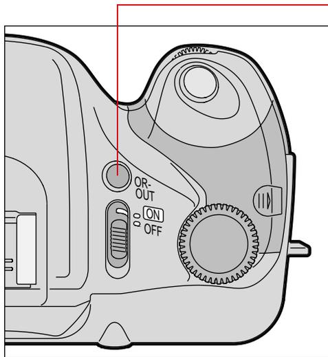
Press and hold the QR-OUT button and rotate the Main-Command dial until your previous memory setting identification number appears. The customized settings appear in the Camera Status LCD panel. Remove your finger from the QR-OUT button. The QR identification number disappears.
