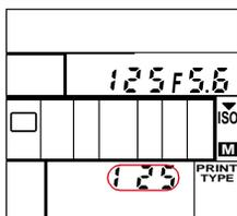
3 Press and hold the SET button and rotate the Main-Command dial until the desired ISO appears in the Camera Status LCD panel and **M** appears. Remove your finger from the SET button to complete the setting.
