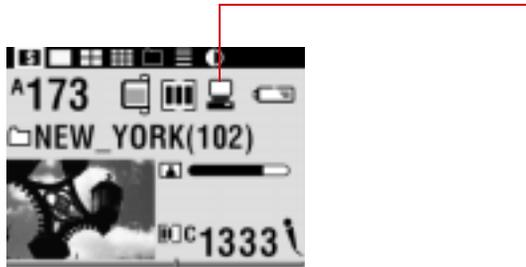
The Host Computer Connected icon on the Status screen appears when a valid cable connection is made. It flashes when a host computer application (such as the Kodak Software) is running.
