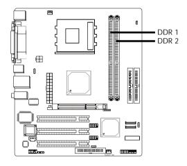
The system board supports DDR SDRAM DIMM. Double Data Rate SDRAM (DDR SDRAM) is a type of SDRAM that doubles the data rate through reading and writing at both the rising and falling edge of each clock. This effectively doubles the speed of operation therefore doubling the speed of data transfer.
