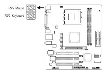
The system board is equipped with an onboard PS/2 mouse (Green) and PS/2 keyboard (Purple) ports - both at location CN1 of the system board. The PS/2 mouse port uses IRQ12. If a mouse is not connected to this port, the system will reserve IRQ12 for other expansion cards.
