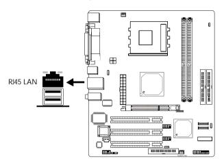
The KM400A-MLV, KM400-MLV and KM400-MLVE system boards are each equipped with an onboard RJ45 fast-ethernet LAN port at location CN6 of the system board. It allows the system board to connect to a local area network by means of a network hub.
