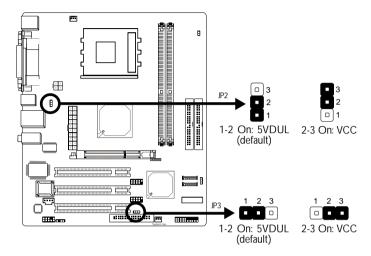
JP2 (USB 1-4) and JP3 (USB 5-8) are used to select the power of the USB ports. Selecting 5VDUL will allow you to use a USB device to wake up a system from the S1 state.
