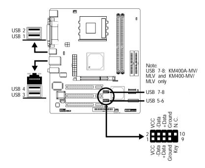
Four onboard USB 2.0/1.1 ports (Black) are at locations CN5 (USB 1-2) and CN6 (USB 3-4) of the system board.
