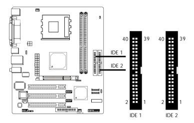
The system board is equipped with two shrouded PCI IDE headers that will interface four Enhanced IDE (Integrated Drive Electronics) disk drives. To prevent improper IDE cable installation, each shrouded PCI IDE header has a keying mechanism. The 40-pin connector on the IDE cable can be placed into the header only if pin 1 of the connector is aligned with pin 1 of the header.
