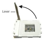
5. Position the CPU above the socket then align the gold mark on the corner of the CPU (designated as pin 1) with pin 1 of the socket.
