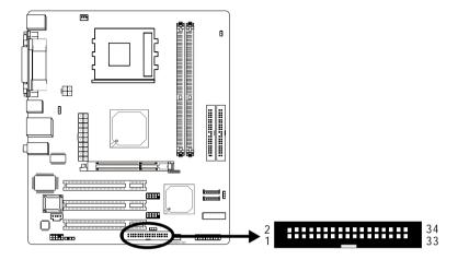
The system board is equipped with a shrouded floppy disk drive connector for connecting a standard floppy disk drive. To prevent improper floppy cable installation, the shrouded floppy disk header has a keying mechanism. The 34-pin connector on the floppy cable can be placed into the header only if pin 1 of the connector is aligned with pin 1 of the header.
