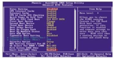
The screen above list all the fields available in the Advanced BIOS Features submenu, for ease of reference in this manual. In the actual CMOS setup, you have to use the scroll bar to view the fields. The settings on the screen are for reference only. Your version may not be identical to this one.
