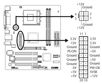
We recommend that you use a power supply that complies with the ATX12V Power Supply Design Guide Version 1.1. An ATX12V power supply has a standard 20-pin ATX main power connector and a 4-pin +12V power connector that must be inserted onto CN9 and CN8 connectors respectively.
