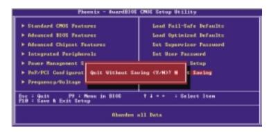
Type "Y" and press <Enter>. The system will reboot and you will once again see the initial diagnostics on the screen. If you wish to make any changes to the setup, press <Ctrl> <Alt> <Esc> simultaneously or <Del> after memory testing is done.
