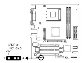
The S/PDIF-out connector (J3) is used to connect external S/PDIF port. The S/PDIF-out port may be mounted on a card-edge bracket. Install the card-edge bracket to the system chassis then connect the audio cable connector to J3. Make sure pin 1 of the audio cable connector is aligned with pin 1 of J3.
