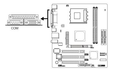
The system board is equipped with an onboard serial port (Teal/Turquoise) at location CN4 of the system board. It is a RS-232C asynchronous communication port with 16C550A-compatible UART that can be used with a modem, serial printer, remote display terminal or other serial devices.
