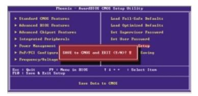
Type "Y" and press <Enter>. The modifications you have made will be written into the CMOS memory, and the system will reboot. You will once again see the initial diagnostics on the screen. If you wish to make additional changes to the setup, press <Ctrl> <Alt> <Esc> simultaneously or <Del> after memory testing is done.
