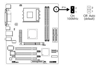
This jumper is used to select the front side bus of the CPU installed on the system board. The default setting is Auto. The system will run according to the front side bus of the CPU installed on the system board. You can also set the FSB fixed at 100MHz by setting JP16 to On.
