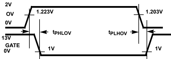
FIGURE 3A. OV TO GATE TIMING
