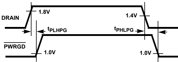
FIGURE 4A. DRAIN TO PWRGD TIMING (ISL6140)
