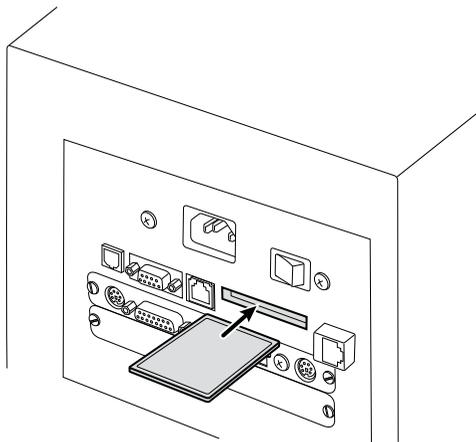
**Installing a Memory Card:** Slide the CompactFlash card into the memory card slot in the rear panel.
