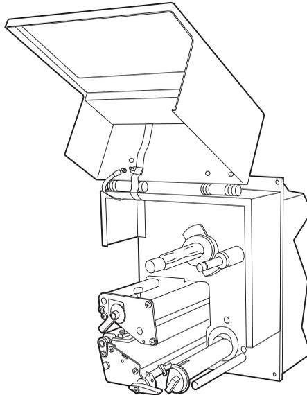
With the access door open, you can easily reach the PA30 print mechanism for setup and maintenance.
