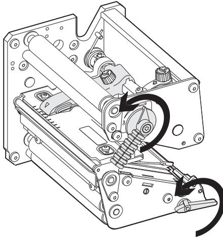
**Opening the Printhead and Pinch Rollers**
