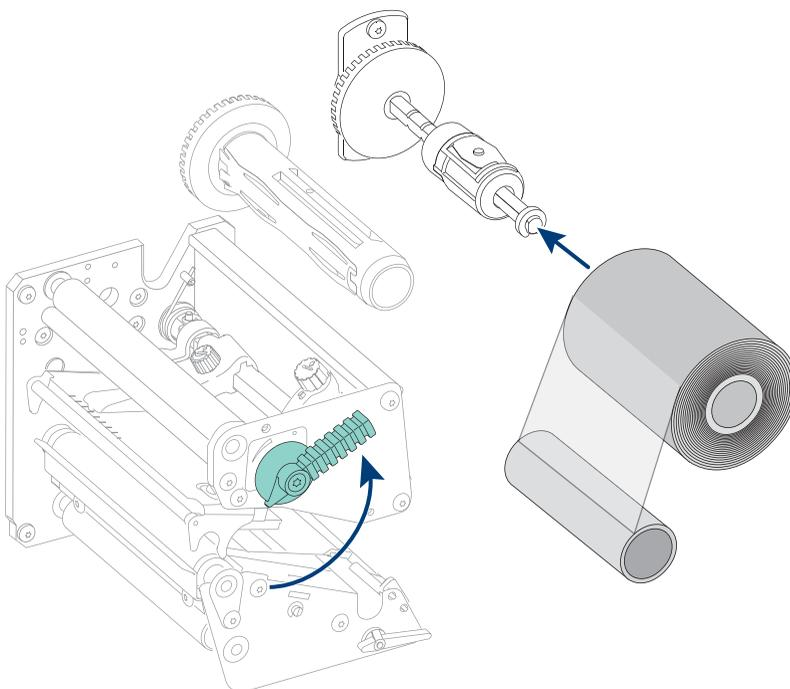
**6** Route the ribbon through the print mechanism. Pull out about 20 cm (8 in) of ribbon.
