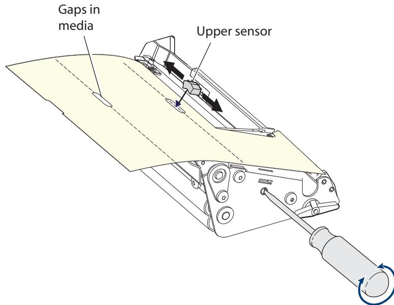
**Positioning the Label Stop Sensor:** Align the center point of the upper sensor with the gaps to be detected. The printhead is omitted here for clarity.
