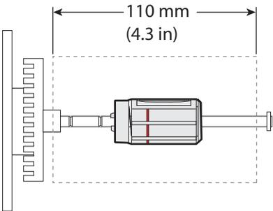
**Bobbin Placement:** *The bobbin should be in the center of the roll of ribbon.*
