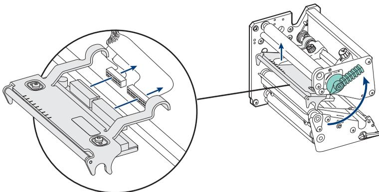
**Replacing the Printhead:** After you pull the printhead out, disconnect the cables.
