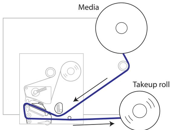
**Media Route:** This illustration of a typical applicator shows the media path through the PA30.
