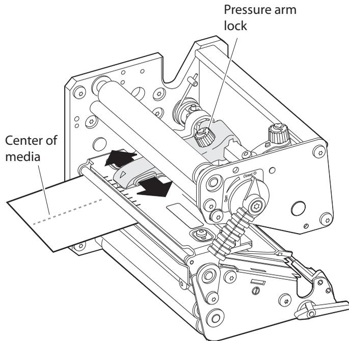
**Pressure Arm Adjustment:** Loosen the pressure arm lock knob and slide the pressure arm until it is centered over the media.
