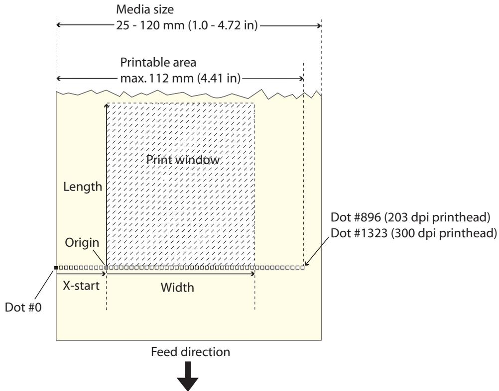
**Print Window Dimensions:** This illustration shows the relationship of the *Xstart*, *Width*, and *Length* settings to the media size and printable area.
