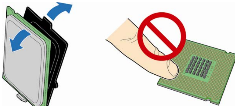
Figure 9. Remove the Processor from the Protective Processor Cover
