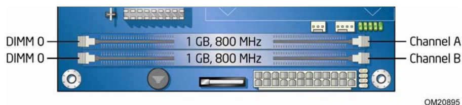
Figure 13. Dual Channel Memory Configuration Example
